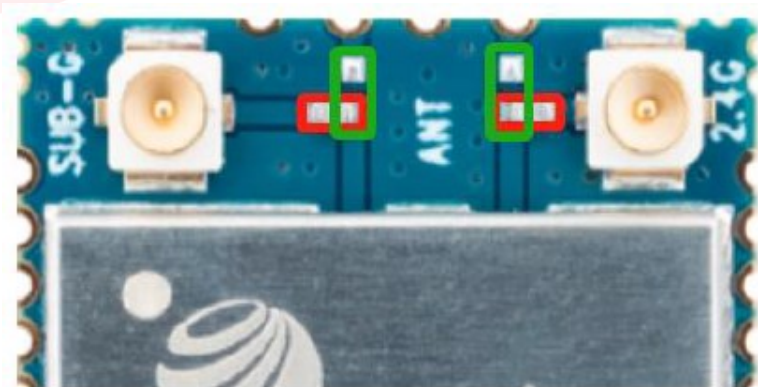
Figure 8. Antenna Output Mode Modification of RF-TI1352P2
